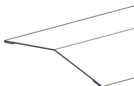
T Wood Roof V Flashing
