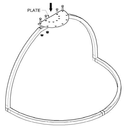
**Step 5:** Attach R2, R3, R4, R5, and R6 to top plate using provided bolts. Use self tapping screws to secure the ribs to LPR and RPR.
