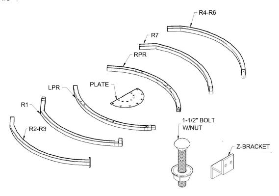
**Step 2:** Connect R1 And R7, and Connect LPR and RPR. You may need a rubber mallet to set the tubing into the fittings. The Velcro will be facing outwards on all above-mentioned parts.
