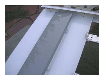
Hook the valance parts of the top pans to the hooks on the apron bar.
