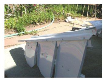
Attach the bottom pans (pans with two rectangular holes) to the flashing with #8-32 x 1/2" bolts and nuts.
