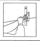
Measure & mark the desired awning location along the wall with a pencil. Use a level to ensure the line is square or measure down from an overhang or header & mark the remaining brackets. The mounting brackets are to be installed on the studs closest to the arm attachments. Note the locations of the Arm Attachments on the Awning's square mounting bar. Then mark their locations on the wall. (Keep brackets clear of these marked locations)
