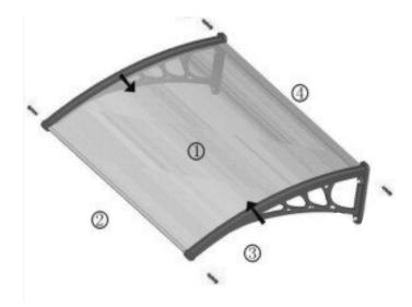
Drive the 4 small screws into the front and back aluminum bars through the holes in the brackets.
