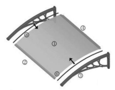
Install the left and right rubber seals. Install the left bracket. It might be easier to align the polycarbonate sheet with the bracket groove if the bracket is lying on the floor and the sheet is in the vertical position. Use a rubber mallet if necessary. Install the right bracket.
