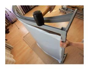
9. Turn the assembly around, install the rubber seal and the second bracket. Drive small screws through the holes in the bracket into the front gutter and back bar (see Step 8).
