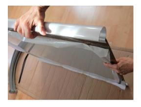
5. Turn the PC sheet around and install a rubber seal on the other long side (see Step 3). Install the front gutter. The open side of the gutter should be on the same side with the non-transparent protective film. It will face up.
