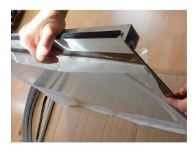
4. Install the back aluminum bar. The flat side of the back bar should be on the same side with the non-transparent protective film. It will face up. Insert the rubber strip into the groove in the back aluminum bar if it is not preinstalled.
