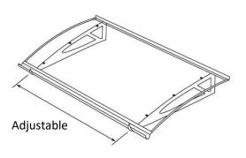
The bracket position along the width of the canopy is adjustable during the assembly. Decide where you want the brackets located relative to the PC sheet.
