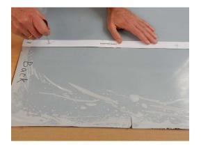
5. Align the edge of the supplied Bracket Hole Template with the bracket line and the Back end of the template with the Back edge of the PC sheet. The template should be located toward the center of the PC sheet. Fix the template in place with adhesive tape. Put a mark for a bracket hole through each of the 3 circles in the template. Repeat for the other bracket.
