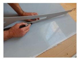
3. Lay the PC sheet on the floor or table with the non-transparent protective film facing up. Put one of the brackets on top of the PC sheet with the bracket holes facing toward the center and make a mark at the outside edge of the bracket. Repeat with the other bracket.
