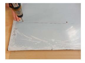
6. Put a piece of wood under the sheet to protect the floor or table. Use a 3/8" drill bit to drill 3 holes for each bracket.
