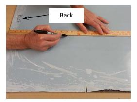
4. Use a ruler to draw bracket lines through these marks parallel to the side edges of the PC sheet. It is important that the lines are parallel to the side edges. Designate one of the sheet edges perpendicular to the lines as Back.
