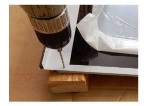
10. Drill a pilot hole in the corner through the back bar and side bar and drive a small screw to fix the side bar inside the back bar. Repeat in the other 3 corners to fix both side bars in the back bar and front gutter.
