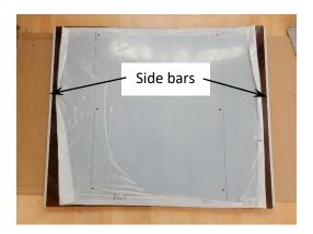
7. Peel the protective film back about 1" from all 4 edges of the PC sheet on both sides. Install the side bars on the PC sheet.
